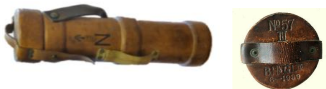
Fig 2. Cordite charges were carried to the gun in flash-proof leather Clarkson cases.
