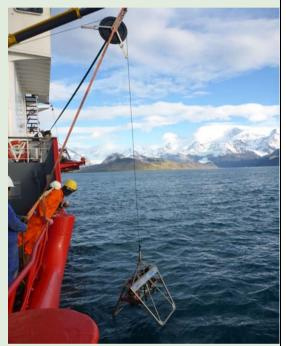
The deep-water camera being deployed from Pharos SG
