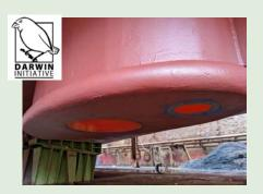
The echousouder transducers fitted to the Pharos SG's hull.
