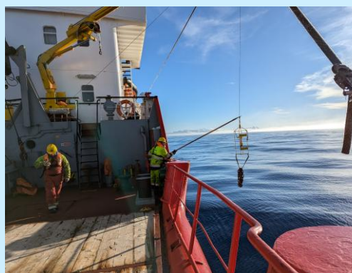
p. 12. CTD (Conductivity, Temperature and Depth) instrument deployment from FPNV Pharos SG (Photo: Jaimie Cleeland)
